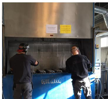
Dippewriter with jacuzzi flushing, liquidfiltration and option of manual spraying.
