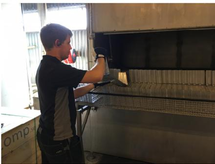
Multi-step spraywasher with interchangeable fixtures to handle different types of goods.
