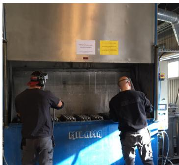
Dippwasher with jacuzzi flushing, liquidfiltration and option of manual spraying.
