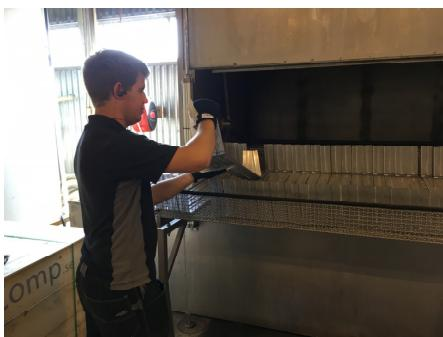
Multi-step spraywasher with interchangable fixtures to handle different types of goods.
