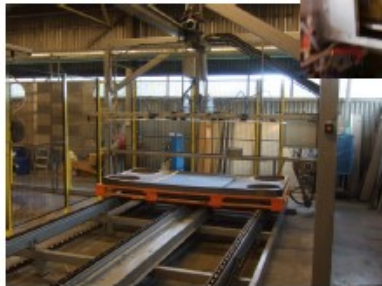
Tunnel washer with chain transport and robotic loading/offloading
