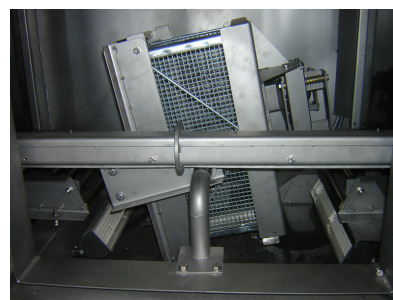
Rotation of basket in cleaning and drying steps. Angle and speed are adjustable.
