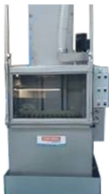
Safety tank under the machine
