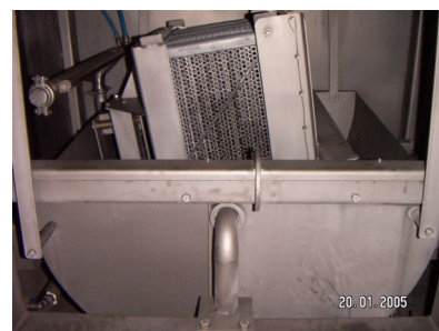
Rotation of basket in cleaning and drying steps. Angle and speed are adjustable.
